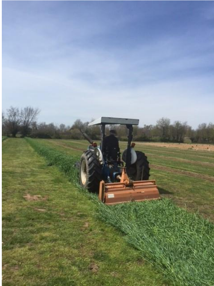
The cover crop was “crimped” using a rototiller with the PTO turned off.
