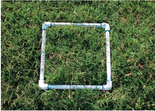
Figure 4. Fall armyworm sampling device.
