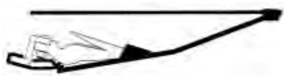
Figure 8-1. Guard extension, usually attached to every other guard, for grain sorghum.
