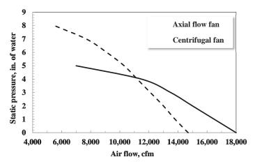
Figure 15-7. Axial and centrifugal fan curves.
