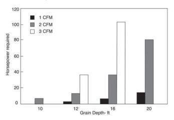
Figure 15-8. Fan power requirements versus depth.
