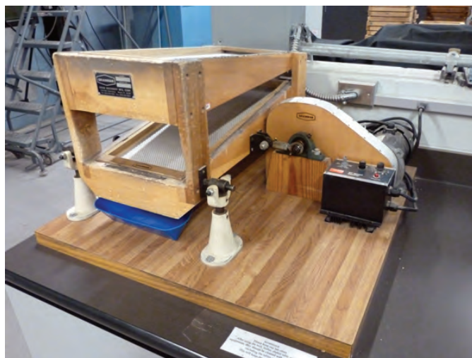
Photo 14-3. A laboratory-scale rice sizing device (Model 61, Grain Machinery Manufacturing Corp., Miami, Florida, USA).
