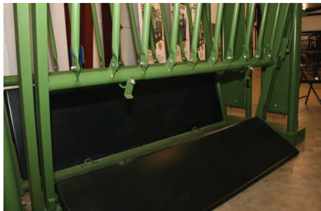
FIGURE 11-3. Lower panels can be removed to access the cattle's feet and legs.
