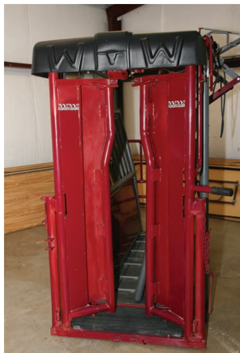
FIGURE 11-1. All controls are on the front of the chute for one-man operation.
