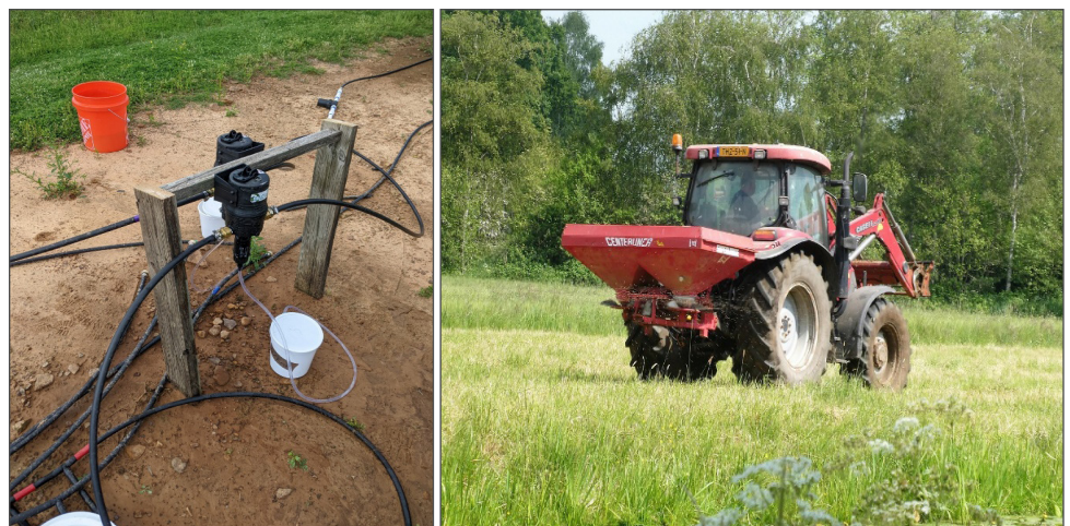
Figure 1. Dosamatic injector (left) used for fertigation. As water moves through the irrigation line (black hose), the Dosamatic draws up a fertilizer solution (white bucket) to be added to the irrigation water that will go through the drip line. Tractor with fertilizer broadcaster (right) spreads granular fertilizer over a wide area of the field.
