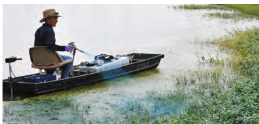
Boat Mounted Sprayer Source: Kelly Duffy, Helena Chemical
