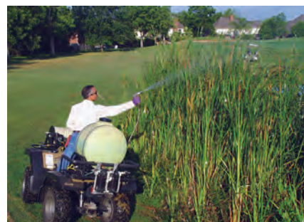
ATV-Mounted Sprayer Source: Kelly Duffy, Helena Chemical
