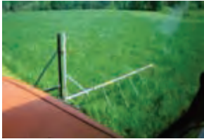
Figure 10. A wildlife flushing bar viewed from inside a tractor cab.
