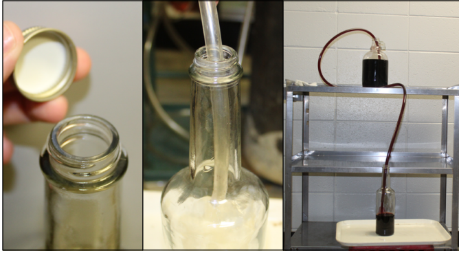
Figure 12. Screw cap and wine bottle (left), sparging a wine bottle with nitrogen gas (center) and bottling wine with gravity siphoning (right)
