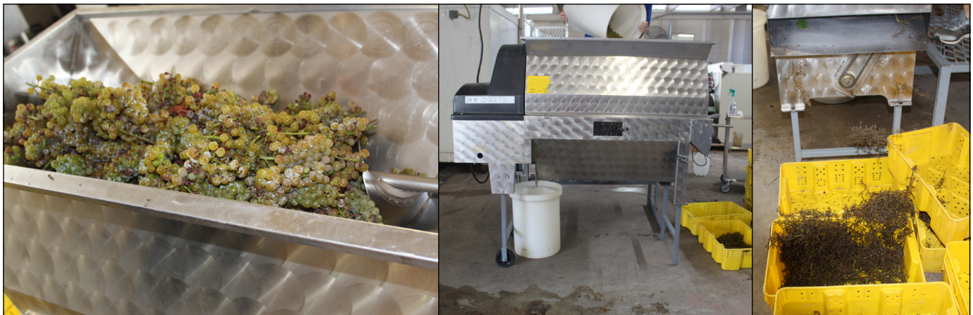
Figure 3. Top view (left), side view (center) and back view (right) of a small-scale commercial grape crusher-destemmer
