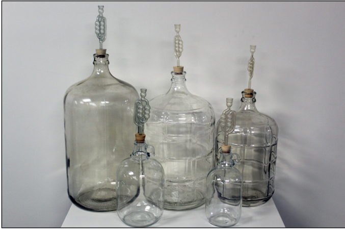
Figure 7. Various sizes from 1.9 L (0.5 gal) to 23 L (6 gal) of glass carboys with fermentation locks used for winemaking
