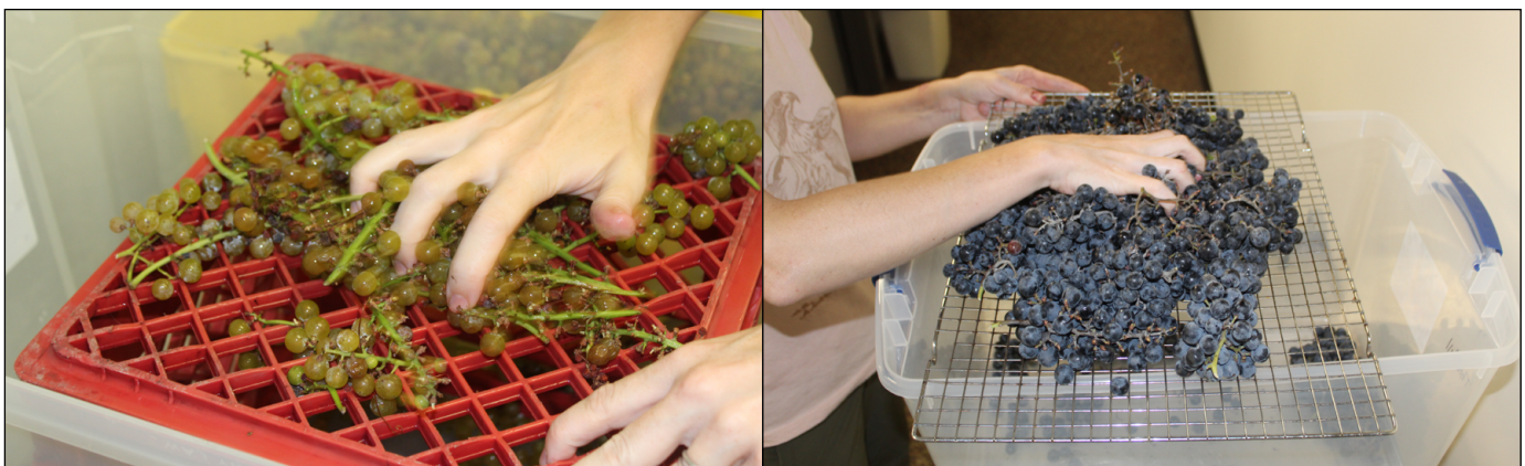
Figure 4. Crushing and destemming grapes in plastic bins using a plastic milk crate (left) or stainless steel baking cooling grid/rack (right)
