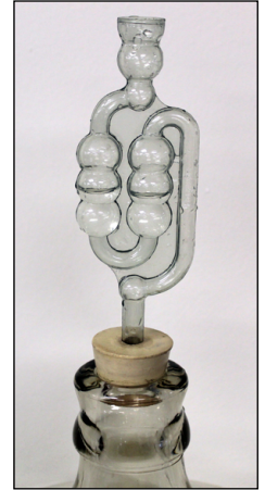
Figure 9. Fermentation lock containing a sulfite solution inserted in a cork on a carboy of wine
