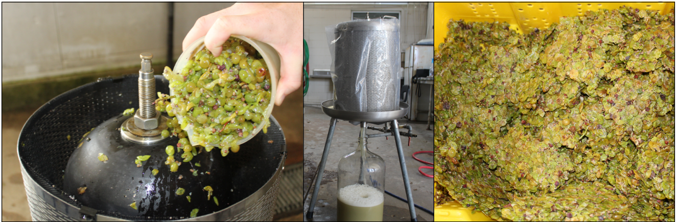
Figure 5. Loading a small-scale commercial vertical grape bladder press (left), pressing the grapes (center) and grape skins/pomace after pressing (right)
