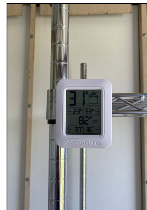
Figure 11. Temperature and humidity reader installed on a wire shelf in walk-in dehydrator (Clarksville, AR).
