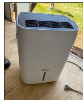
Figure 12. A 50-pint dehumidifier set up in the walk-in dehydrator (Clarksville, AR).
