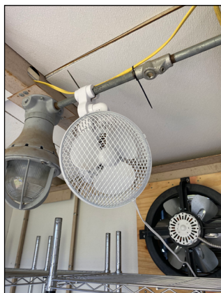
Figure 10. Clip-on oscillating fan installed in walk-in dehydrator (Clarksville, AR).
