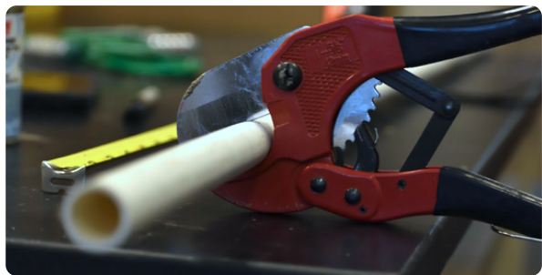
Figure 2. Use PVC pipe cutter to get the desired lengths.
