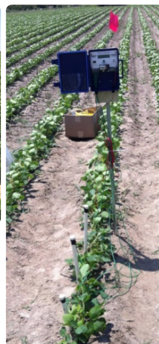
Figure 3. Sensors should be installed early in the season when plants are small so that the installation does not damage roots. Plants with roots that are damaged by sensor installations may not use water the same as undamaged plants.
