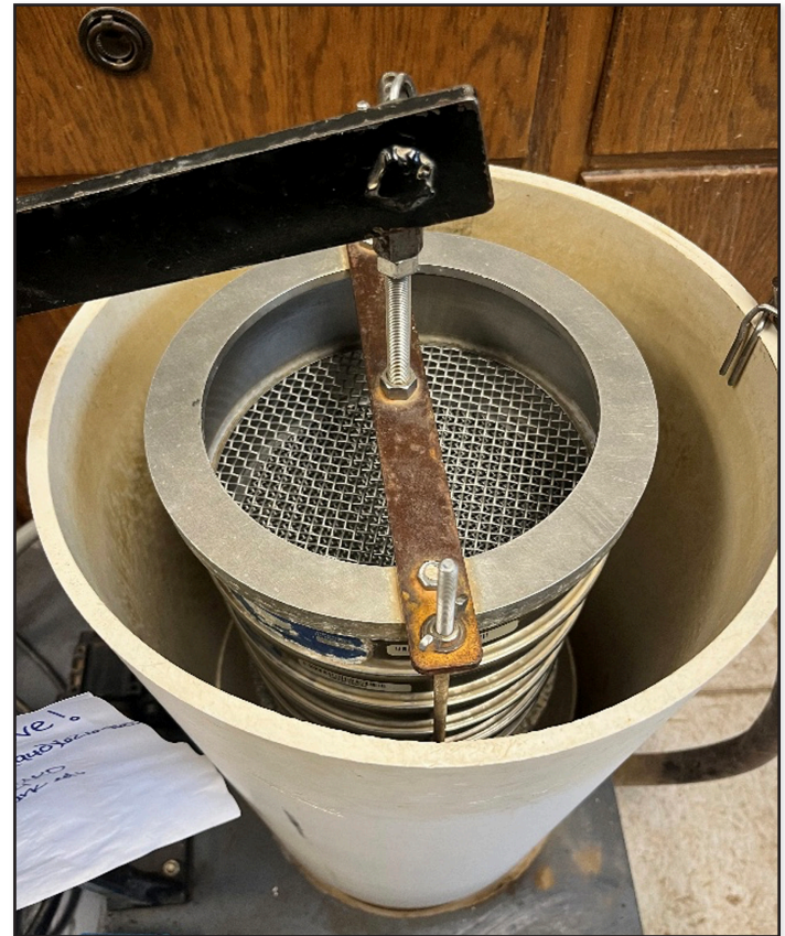
Figure 4: Wet-sieve apparatus that utilizes five sieves of gradually increasing mesh count that are submerged in water and mechanically agitated by raising and lowering continuously.
