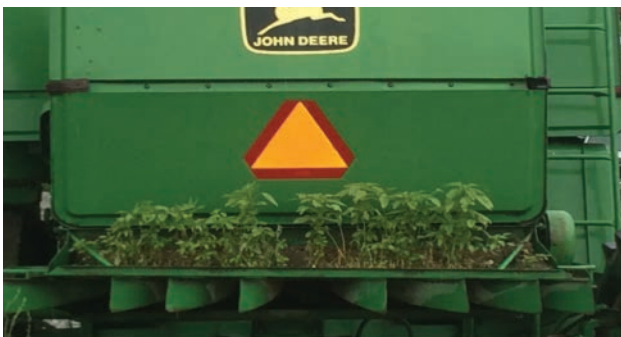
Figure 6. Palmer amaranth seed can contaminate many areas of harvesting equipment. Clean equipment often to prevent spread.
