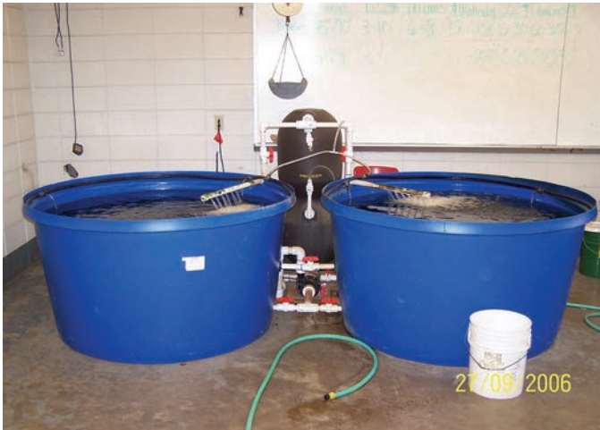
FIGURE 1. A two-tank system composed of two 500-gallon polypropylene tanks, a 1/8-hp pump and a bead filter.
