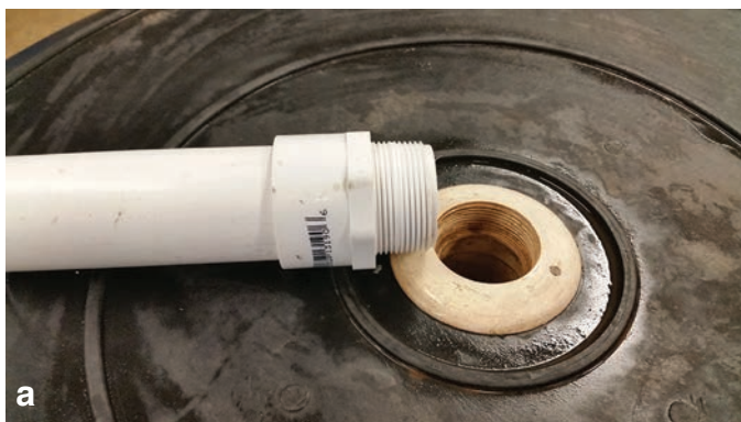
FIGURE 2. Sealing a leak between threads inside a bulkhead fitting. 2a: threads to be sealed; 2b and c: applying silicone sealant; 2d: threading complete, note the bead of silicone formed between the bulkhead and the pipe joint.
