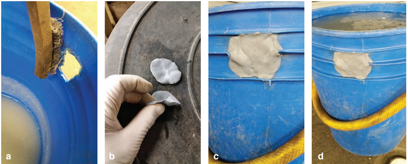
FIGURE 7. Using epoxy putty to repair a 1-inch diameter hole. 7a: Follow plastic and putty preparation instructions in Figure 5; 7b: make two thin discs and apply one to each side of the wall; 7c: this will create a wall that will set and be impervious to water, 7d.
