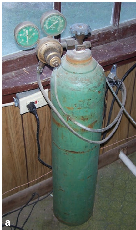
FIGURE 10. A solenoid valve (cube in b.) and oxygen tank can be a useful combination for oxygen backup. The solenoid valve is plugged into an electric receptacle (a.) which keeps the valve closed. In the event of a power outage, lack of electricity opens the valve and oxygen can flow to the fish. The tank should be well secured and all fittings in good condition to ensure oxygen does not leak from the system. Although this setup has a regulator, it does not include a flow meter, which is preferable.
