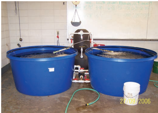
FIGURE 1. A two-tank system composed of two 500-gallon polypropylene tanks, a 1/2-hp pump and a bead filter.
