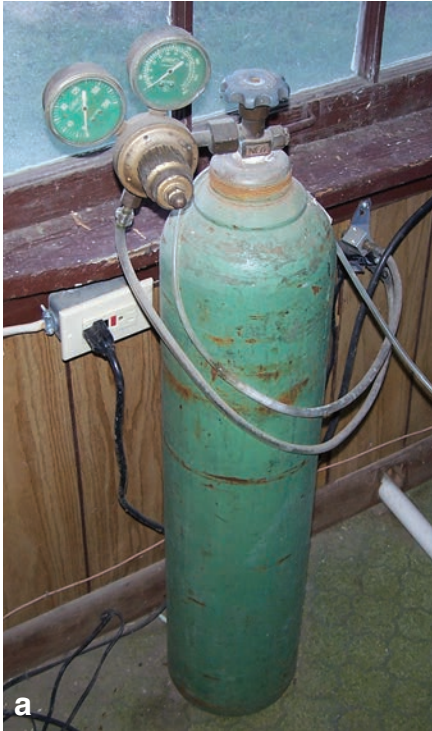
FIGURE 10. A solenoid valve (cube in b.) and oxygen tank can be a useful combination for oxygen backup. The solenoid valve is plugged into an electric receptacle (a.) which keeps the valve closed. In the event of a power outage, lack of electricity opens the valve and oxygen can flow to the fish. The tank should be well secured and all fittings in good condition to ensure oxygen does not leak from the system. Although this setup has a regulator, it does not include a flow meter, which is preferable.
