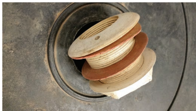
FIGURE 4. Frequently, a bulkhead fitting is equipped with one gasket, but if leaking persists, a gasket may be used on both sides of the wall.
