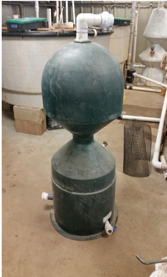
FIGURE 4. Left, a bead filter on its stand with four visible ports. Right, the same filter off the stand, with a better view of the ports.
