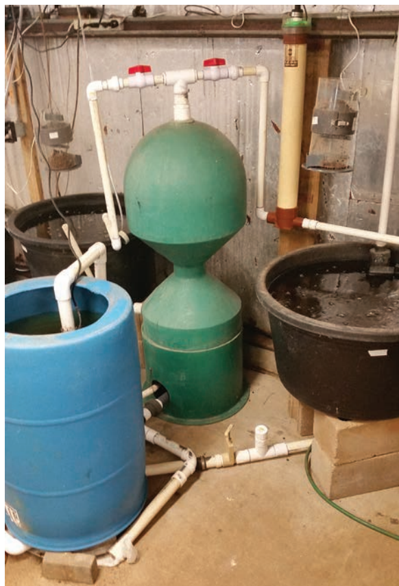
FIGURE 3. Two bead filters with slightly different shapes. Note the 2-inch top ports for water outflow, the 1½-inch drain ports at the bottom, the air-sucking side ports with the one-way check valve and the small 1-inch flash drain. The filter in the top photo uses a check valve on the exit port while the filter in the bottom photo uses manual valves. Backwashing this filter requires closing both valves.
