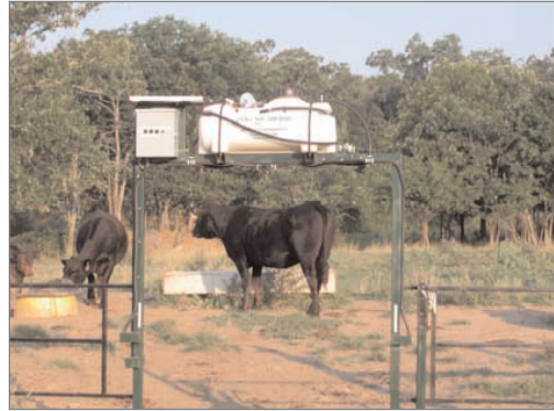
Figure 9b. Solar-powered automatic sprayer.
