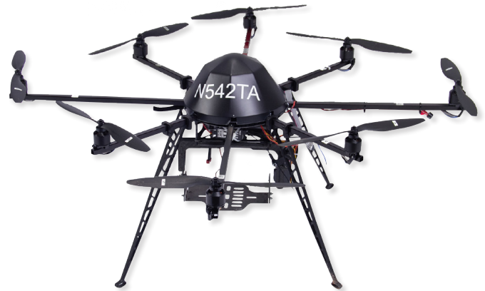
Example of sUAS registration number prominently displayed on the aircraft.
