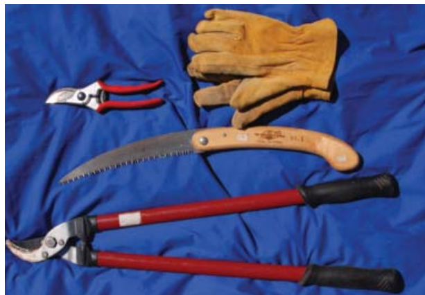
FIGURE 13. Common tools for shrub pruning include a lopper, a by-pass hand pruner, a curved blade/keyhole-type saw and a nice pair of leather gloves.
