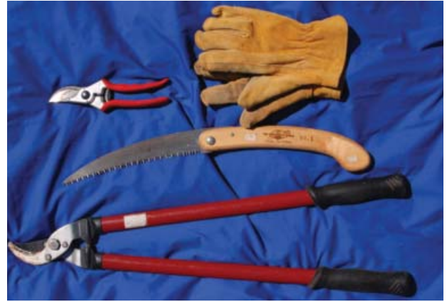
FIGURE 13. Common tools for shrub pruning include a lopper, a by-pass hand pruner, a curved blade/keyhole-type saw and a nice pair of leather gloves.
