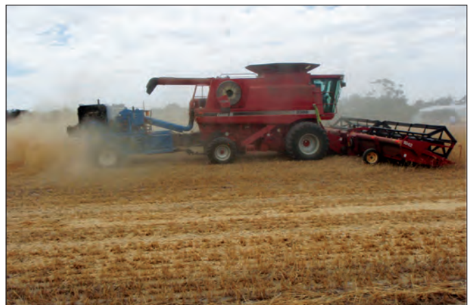
Figure 4. Harrington Seed Destructor used during wheat harvest.
