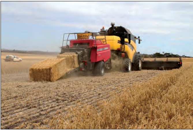
Figure 5. Bale-direct system in wheat.
