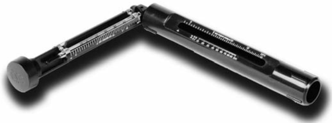
Figure 4. A photo of a sling psychrometer
