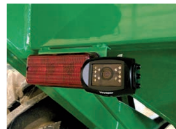
Figure 5. Backup camera mounted on the rear of a grain wagon.
