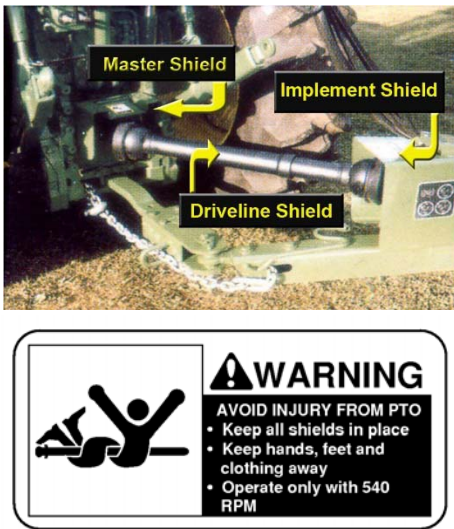
Figure 3. Properly guarded PTO driveline and wrap-up point sign.
