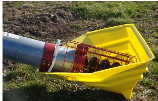
Figure 5. Mechanical guard at inlet of portable grain auger.
