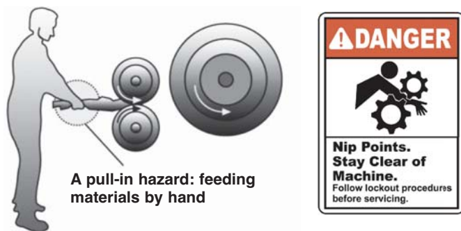
Figure 4. A pull-in hazard resulting from feeding materials into a machine by hand and a nip points sign.
