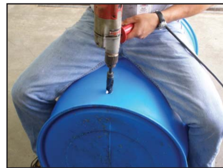
Drilling overflow hole
