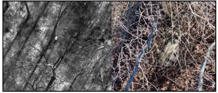
Figure 6. Detection from Matrice 300 UAS with H20T sensor demonstrating heat reflectance from a feral hog in center compared to surroundings (left) and zoomed-in optical image of same feral hog (right).
