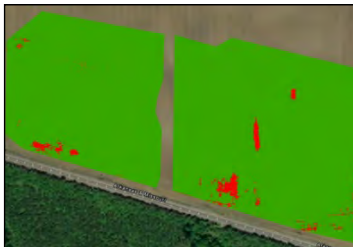
Figure 4. Classified NDVI of two pastures with red indicating feral hog damages.
