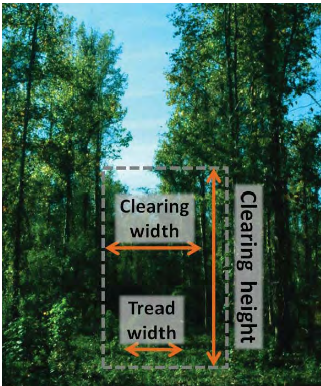
FIGURE 7. Tread width, clearing width and clearing height. Text by the authors, photo by Brian Lockhart, USDA Forest Service, Bugwood.org.
