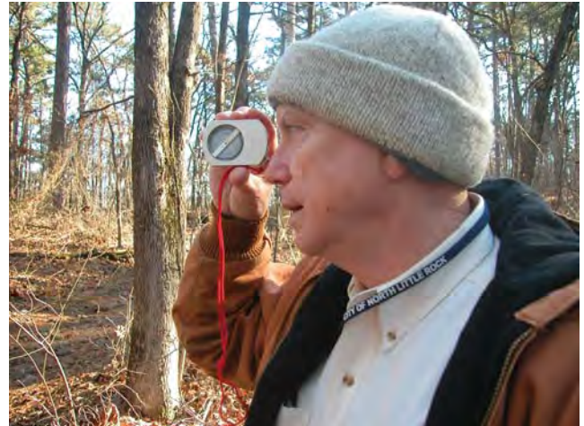
FIGURE 10. A clinometer is a useful tool for evaluating trail grade. Photo by Becky McPeake, UA Division of Agriculture, Cooperative Extension Service.
