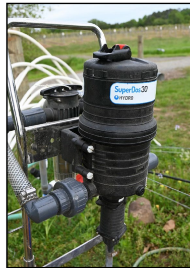
Figure 7: A Dosatron injector pump, a type of positive displacement metering pump.
