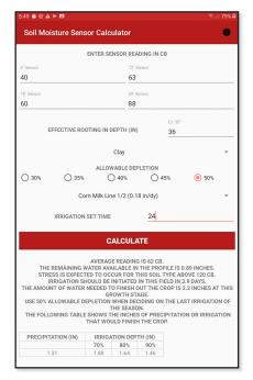
**Figure 2.** Android version of Arkansas Soil Moisture Sensor Calculator result for the example. The app does all of the calculations except adjusting for rainfall. The app can be downloaded at the Google Play Store.
