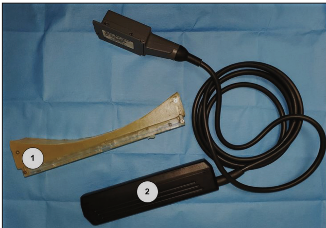
Figure 5. Accessories for the collection of carcass images: 1 – Standoff pad for attachment to ultrasound probe for collection of ribeye image; 2 – A 3.5 Mhz linear ultrasound probe, commonly used in the collection of beef carcass measurements.
