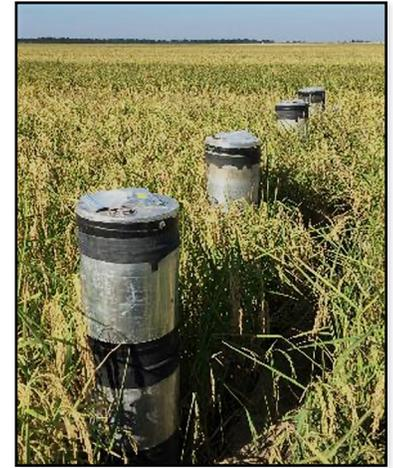
**Figure 2. Greenhouse gas emissions field research set-up for furrow-irrigated rice, out-fitted with 30-cm diameter chambers, sensors, and a data logger to continuously measure and record soil temperatures and soil oxidation-reduction (redox) potentials at one site position in a production-scale field (left panel). Greenhouse gas chambers with caps and extenders to accommodate growing rice later in the growing season (right panel).**
