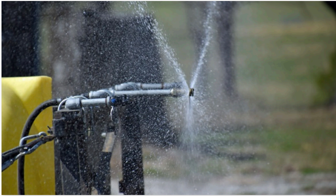
Figure 1. 180° spray pattern of boom-less nozzle.
