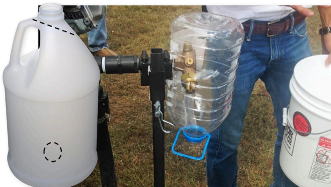
Figure 2. (left) Deflector used in catch test. Figure 3. (right) Secure deflector to nozzle.
