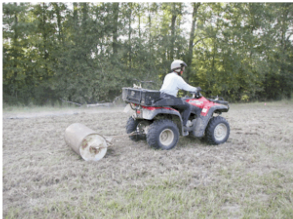
Figure 2. After broadcasting seed, a roller firms the soil around the seeds, ensuring shallow seed placement and seed-to-soil contact.
