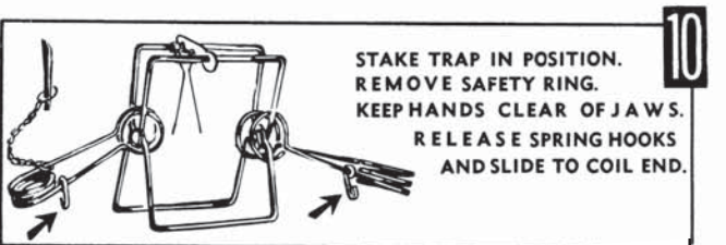
Figure 9. Illustration of how to set a Conibear trap.
