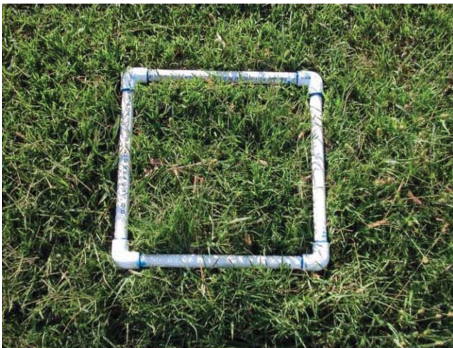
Figure 12. Homemade PVC sampling device for counting armyworms in one square foot of area.
