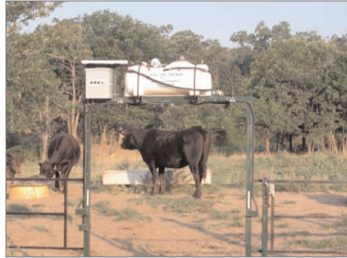
Figure 9b. Solar-powered automatic sprayer.
