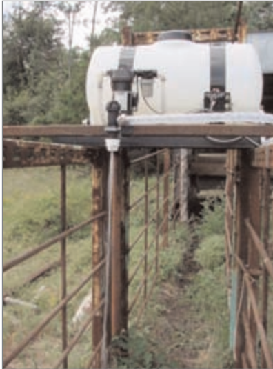
Figure 9a. Battery-powered automatic sprayer.
