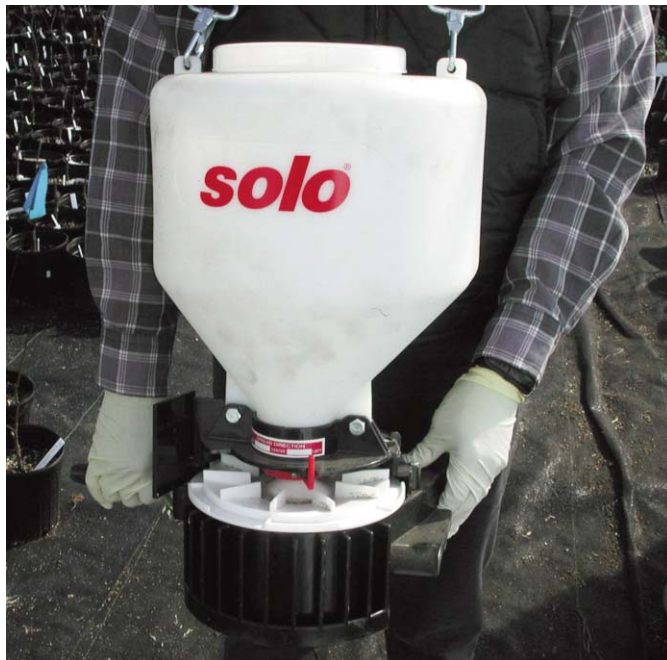
Typical belly-grinder applicator for granular herbicides
