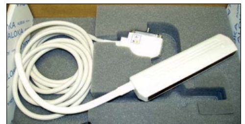
Figure 2. A 3.5 Mhz linear ultrasound probe, commonly used in the collection of beef carcass measurements.
