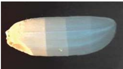
FIGURE 4. Fissured kernel due to rapid moisture adsorption.
