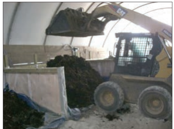
Figure 3. Biodrying pile preparation.
