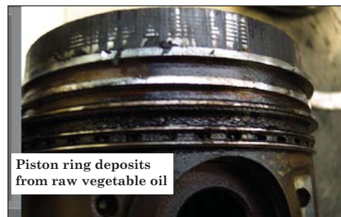
Figure 2. Deposits from raw vegetable oil
