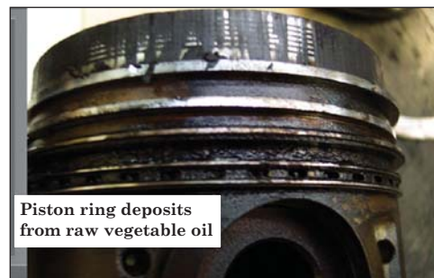
Figure 2. Deposits from raw vegetable oil
