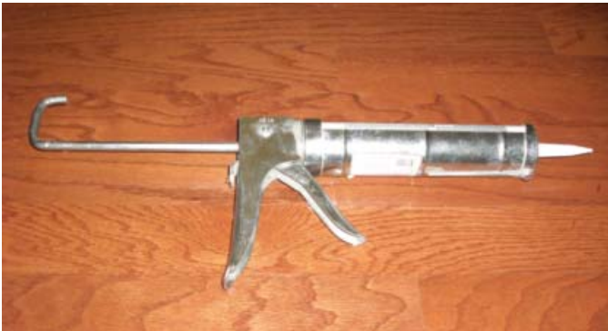
Figure 2. Caulking gun with caulk tube
