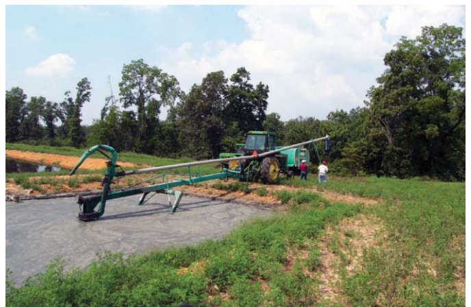
Figure 4. Lagoon agitation pump with load pipe and tank spreader in the background.
