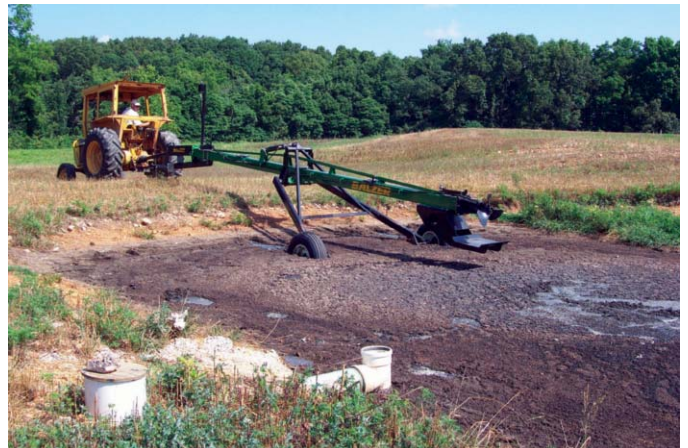
Figure 3. Trailer-mounted prop agitator with mid-size tractor.
