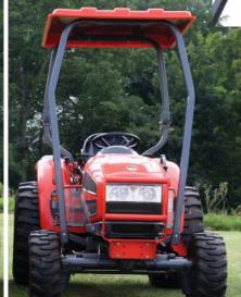
Figure 4. A tractor with a 2-post ROPS outfitted with a FOPS canopy. Horizontal steel supports and vertical steel posts provide additional structural support for the FOPS.
