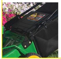
the bag. The bag is subject to wear and deterioration; check the bag frequently and replace when necessary.
