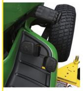
Interlock system assures engine will not start unless mower blades are turned off, brake is on, and traction drive is disengaged.
