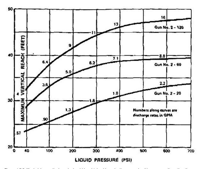
Figure 1.7.5. Maximizing vertical reach should be obtained by selecting a nozzle of larger capacity, rather than increasing the pressure.
