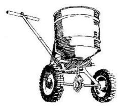
Figure 1.7.3. Centrifugal spreader.
