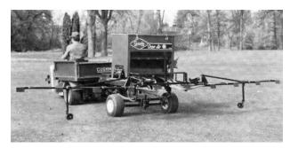
Figure 2.7.5. Example of air spreader.
