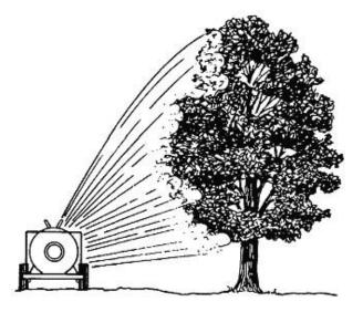
Figure 1.7.6. Air-carrier sprayer used on tall trees.
