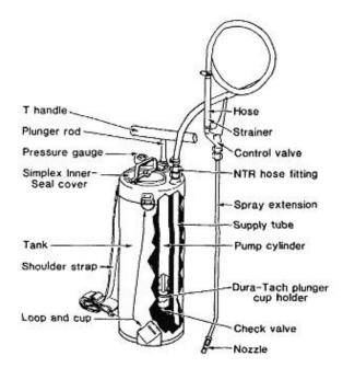
Figure 1.7.1. Compressed air sprayer.
