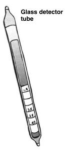
Glass detector tubes are "fumigant specific." That means you will need to purchase a different set of tubes for each type of fumigant you use. Their operation is simple. Place one tube in the area you wish to test. Break the seal. A sample pump will draw a measured amount of air through the tube. A color reaction will occur indicating the fumigant concen-
