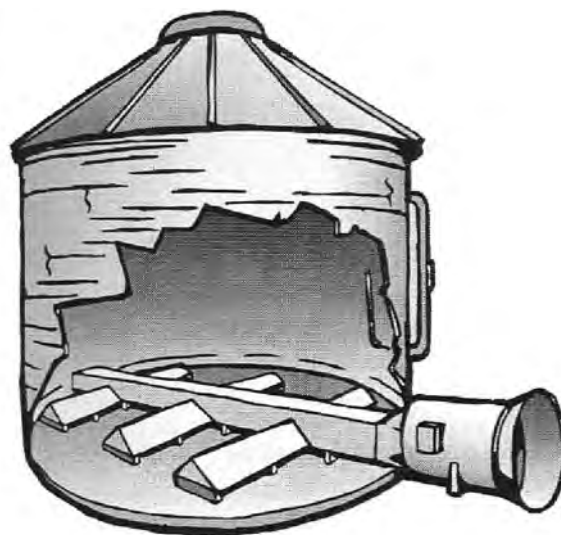
Grain storage recirculation system
