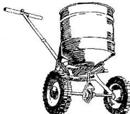
**Figure 1.7.3.** Centrifugal spreader.
