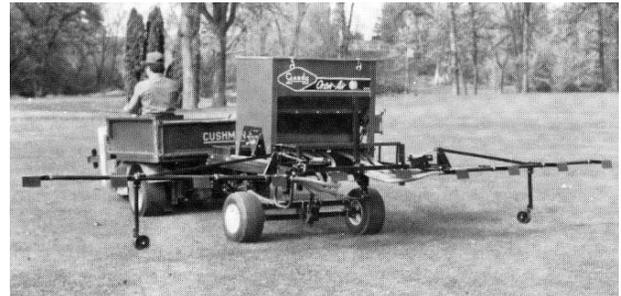
**Figure 2.7.5.** Example of air spreader.
