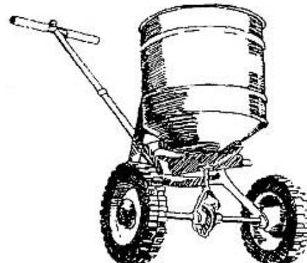
**Figure 1.7.3.** Centrifugal spreader.
