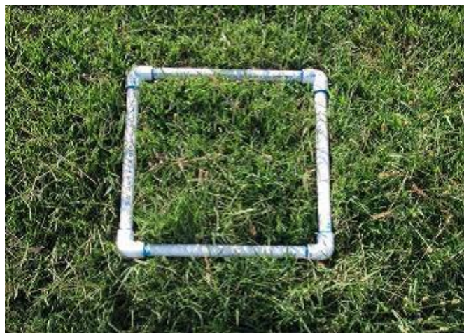
Device used to sample fall armyworm (size: 1 square foot constructed from \frac{1}{2} inch PVC pipe).half-inch PVC pipe).
