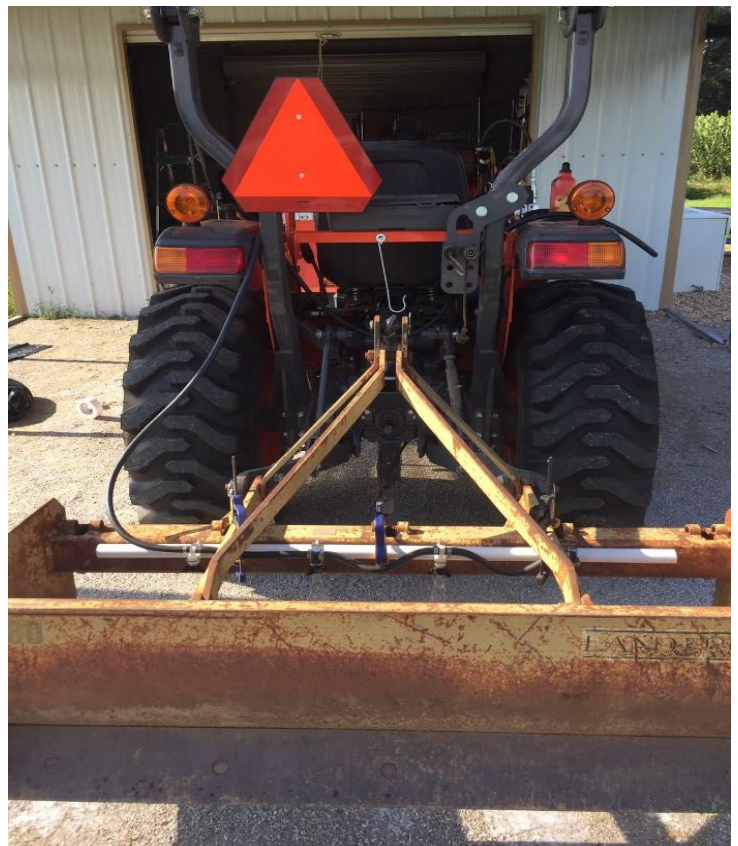
Below right: 4 nozzle boom inside box blade
