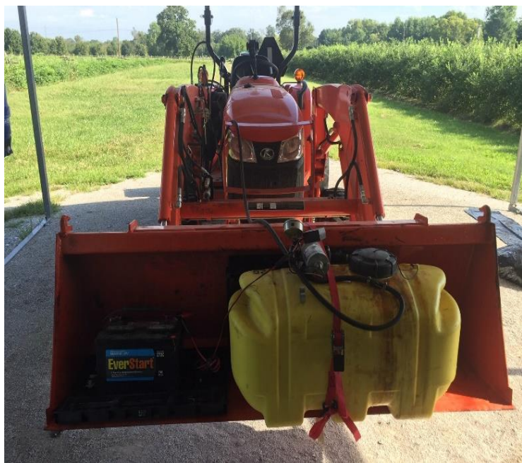
Below: 25gal sprayer inside front end loader
